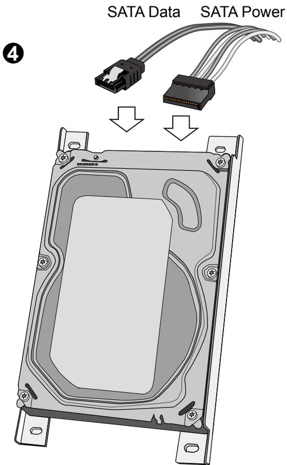
5. Secure the hard disks to the mounting positions in the chassis with its label side facing up, and the connectors facing the inside of the chassis.
