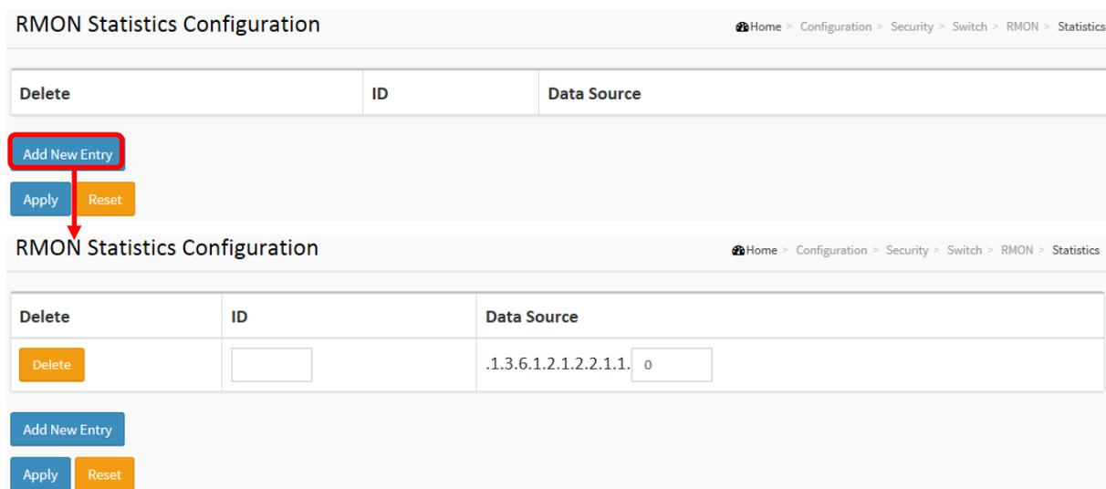
The screenshot shows two instances of the 'RMON Statistics Configuration' page. The top instance shows the 'Add New Entry' button highlighted with a red box and an arrow pointing to the configuration table below. The bottom instance shows the configuration table with a single entry.
