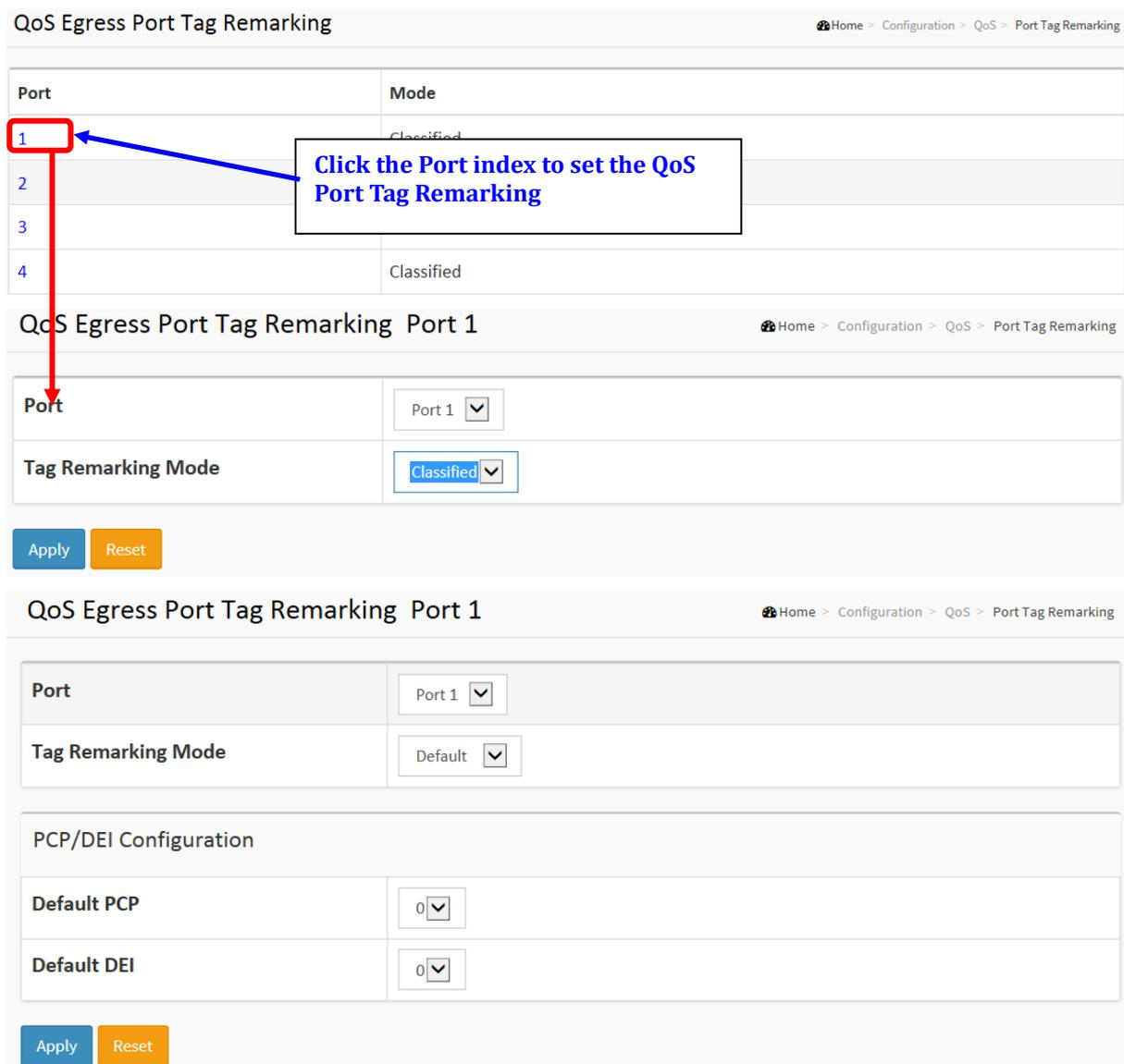
The screenshot illustrates the web interface for configuring QoS Egress Port Tag Remarking. It is divided into three main sections:
