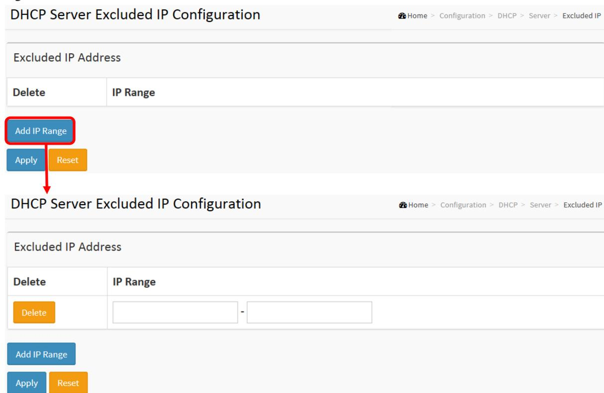
The figure displays two screenshots of the DHCP Server Excluded IP Configuration web interface. The top screenshot shows the 'Add IP Range' button highlighted with a red box, and a red arrow pointing to the 'Apply' button. The bottom screenshot shows the 'IP Range' input field with a 'Delete' button next to it.
