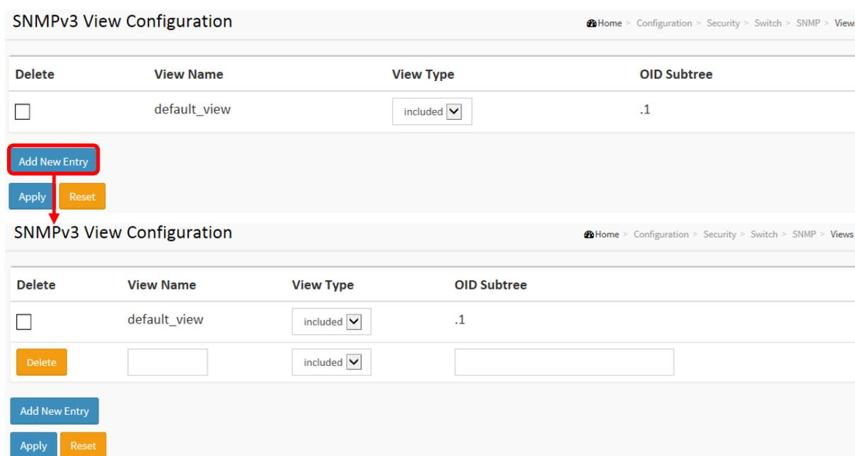
The figure shows two screenshots of the 'SNMPv3 View Configuration' web interface. The top screenshot displays a table with one entry: 'default\_view' with a View Type of 'included' and an OID Subtree of '.1'. A red box highlights the 'Add New Entry' button, with an arrow pointing to the bottom screenshot. The bottom screenshot shows the same interface but with a second empty row for adding a new view, and the 'Add New Entry' button is now blue.
