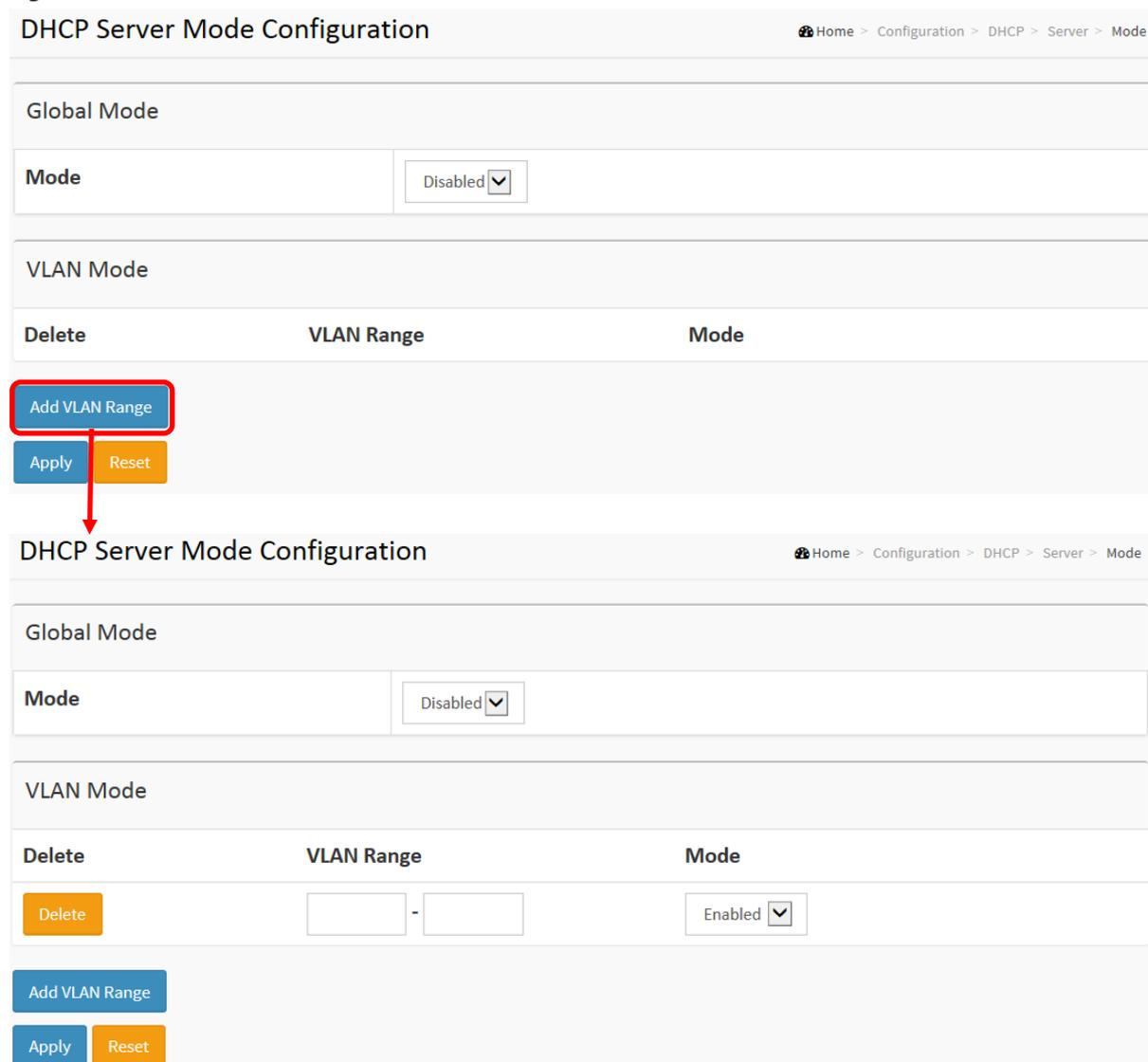
The figure shows two screenshots of the DHCP Server Mode Configuration web interface. The top screenshot shows the 'Global Mode' set to 'Disabled'. A red box highlights the 'Add VLAN Range' button, with a red arrow pointing to the bottom screenshot. The bottom screenshot shows the 'Global Mode' set to 'Enabled' and a new VLAN range added to the table.
