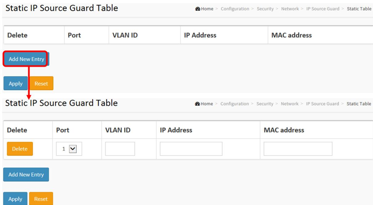
The figure shows two screenshots of the web interface for the Static IP Source Guard Table. The top screenshot shows the 'Add New Entry' button highlighted with a red box and an arrow pointing to the 'Apply' button. The bottom screenshot shows the table with one entry: Port 1, empty VLAN ID, IP Address, and MAC address fields.
