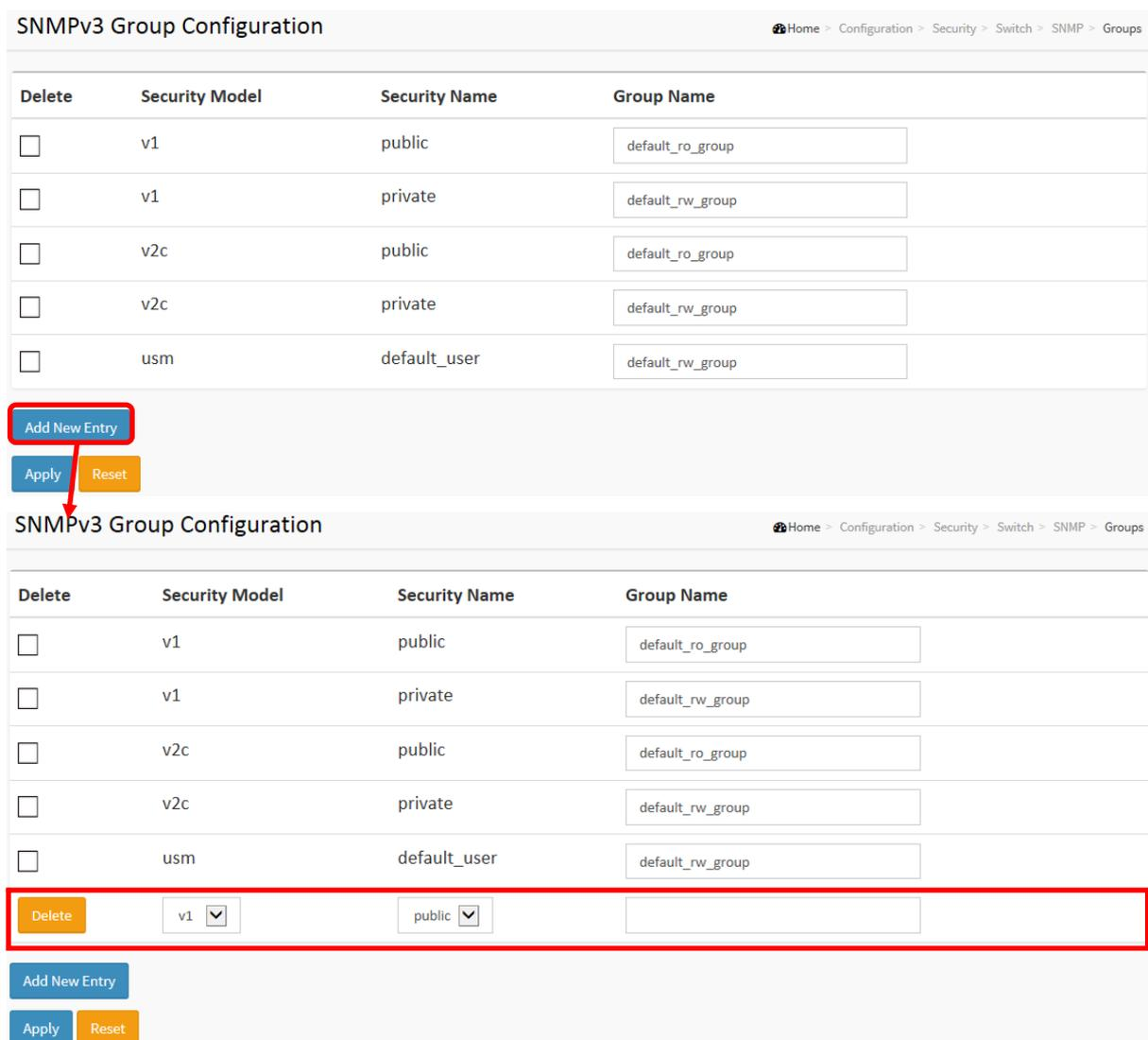
The screenshot shows the 'SNMPv3 Group Configuration' page. It features a table with columns for 'Delete', 'Security Model', 'Security Name', and 'Group Name'. Below the table are buttons for 'Add New Entry', 'Apply', and 'Reset'. A red box highlights the 'Add New Entry' button in the first screenshot and the 'Delete' button, 'Security Model' dropdown, and 'Security Name' dropdown in the second screenshot.
