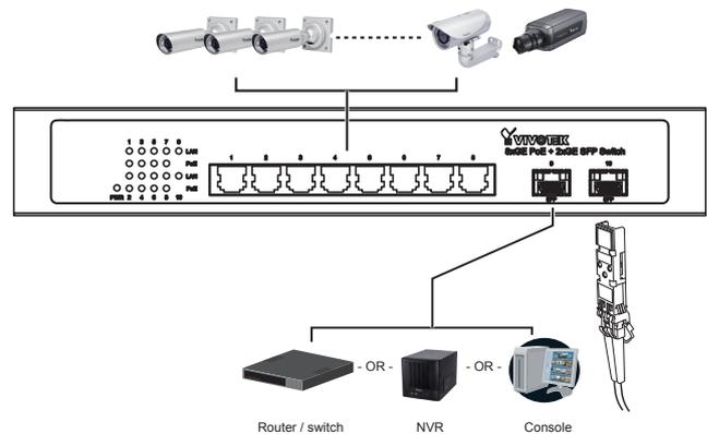
Use SFP, LC type transceiver with GbE transfer speed in Single mode (10km,30km,50km,80km) or Multi mode (0.5m or 2km) or Bidi (10km,30km,50km,80km).
