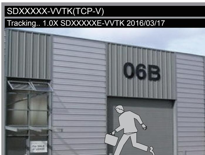
Auto tracking is configured by designating the minimum object size. Moving objects that enter the current region of view will trigger the tracking action.
