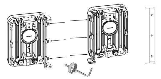
3. Secure two illuminators to sides of B05 mounting bracket, each using 4 M6 socket screws.
