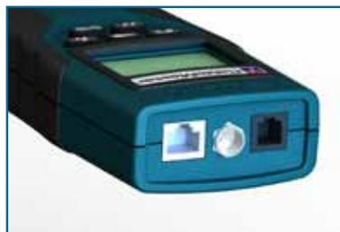
The CableMaster 450 can measure additionally the length of cables.
