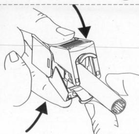
Close up the wings toward each other and push down both sides for secure connection.
