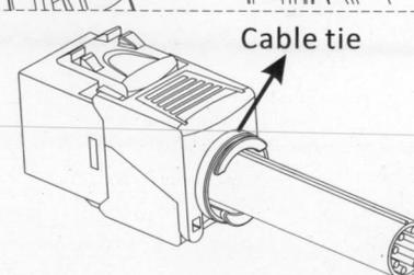
Wrap the drain wire around the shielded holder and tie up the cable.
