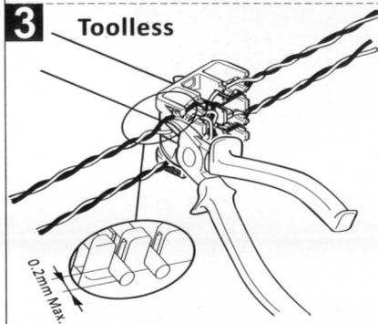
Insert the wires through the cap and seat the wires in the correct slots according to T568A or T568B. Trim the wires flush with the cap. It's recommended the tip of wires is not more than 0.2mm.
