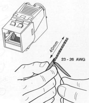
Strip approximately 40mm of the cable jacket. Cut off the plastic cross and separate the wire into 4 pairs.
