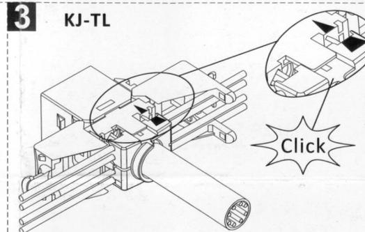
Insert the wires through the cap and seat the wires in the correct slots according to T568A or T568B. Match with the black triangle and align the cap with IDC until it clicked as shown.
