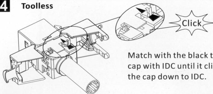
Match with the black triangle and align the cap with IDC until it clicked as shown. Press the cap down to IDC.
