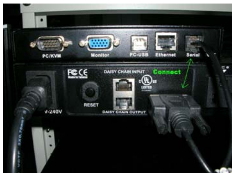
A real connection case of TK-RP08 and TK-IP101
