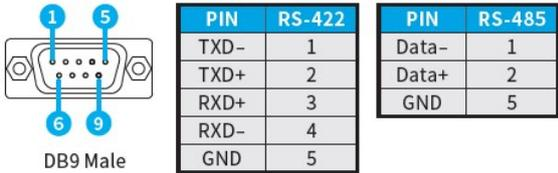
DB9 Female to 5-pin Terminal Block Adapter
