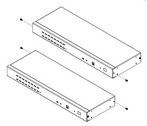
2. Screw the mounting brackets into the sides of the unit at the front or the rear, as shown in the diagram below.
