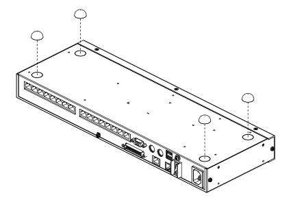
**Note:** To ensure adequate ventilation, allow at least 5.1 cm on each side, and 12.7cm at the back for power cord and cable clearance.
