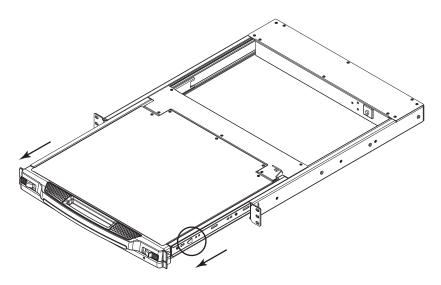
**Note:** The reason for the two step procedure is to minimize the chances of you pinching your fingers when sliding the module in.
