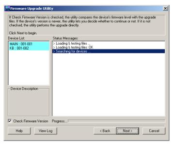
The Utility inspects your installation. All the devices capable of being upgraded by the package are listed in the *Device List* panel.
