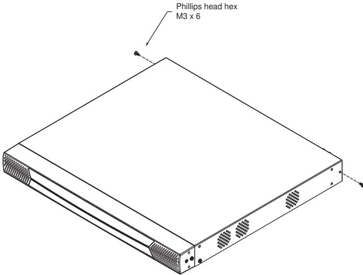
2. Use the M3 x 8 Phillips head hex screws supplied with the rack mount kit to screw the mounting brackets into the rear of the unit.
