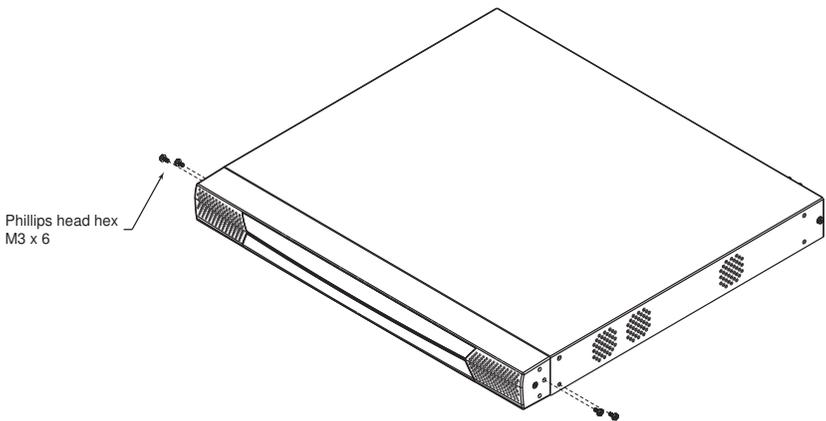
2. Use the M3 x 8 Phillips head hex screws supplied with the rack mount kit to screw the mounting brackets into the front of the unit.
