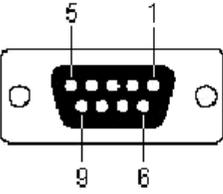
The diagram shows a DB9 Female connector with a 3x3 grid of pins. Pin 5 is at the top-left, pin 1 is at the top-right, pin 9 is at the bottom-left, and pin 6 is at the bottom-right. The connector is labeled "DB9 Female" below it.
