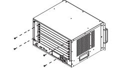
3. Slide the VM7904 into any of the Input Board Slots (4 upper slots) on the Modular Matrix Switch until it secures in place.
