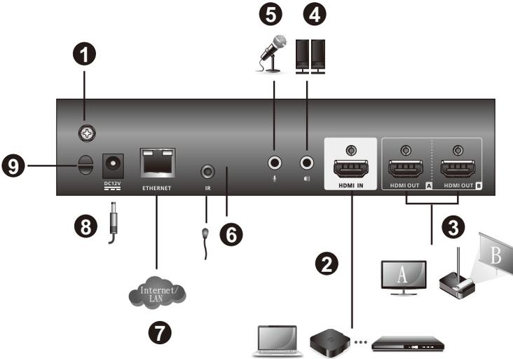
1. Use a grounding wire to ground the unit by connecting one end to the grounding terminal, and the other end to a suitable grounded object.
