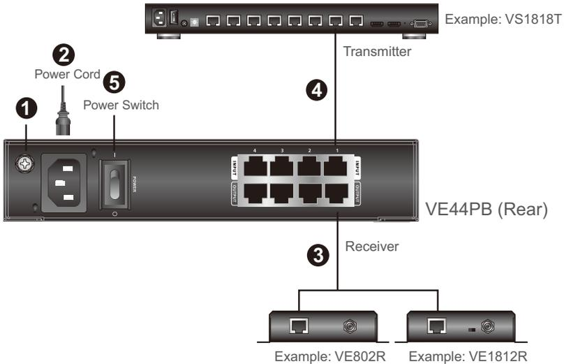
1. Ground the VE44PB by connecting one end of a grounding wire to the grounding terminal and the other end to a suitable grounded object.
