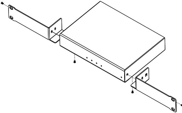
3. Screw the mounting brackets to the rack.
