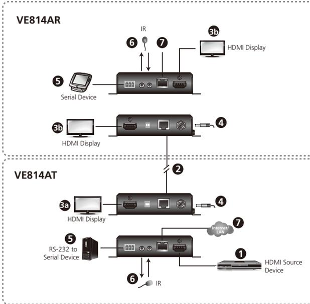
1. Use an HDMI cable to connect the HDMI Out port on your source device to the HDMI In port on the VE814AT.
