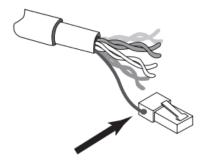
2. The second method is to use the STP cable shielding for grounding. In this case, make sure that the shielding makes tight contact with the inside of the RJ-45 connector, at its top, as shown here:
