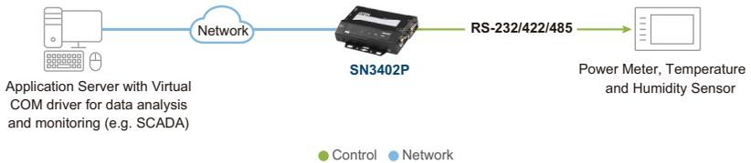
This mode is useful with devices such as POS terminals, bar code readers, serial printers, etc. since it allows users to use software that was written for pure serial communication applications.
