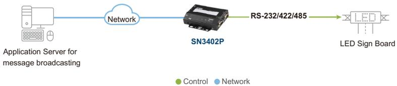
Because it doesn't perform error checking in the thorough way that TCP does, UDP is more suitable for real time applications (such as message display) than the slower TCP, which is optimized for data accuracy.
