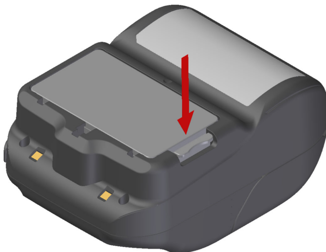
Figure 8-4 Installing Battery Pack (2)
