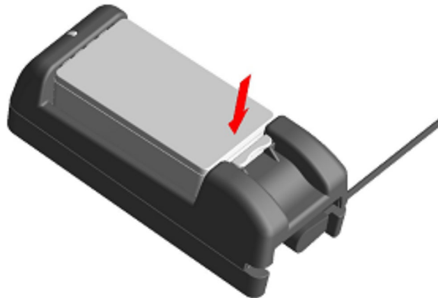
Figure 19-6 Installing Battery Pack (2)
