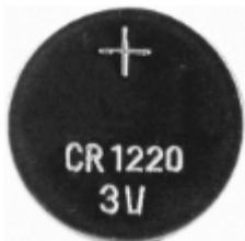
5. Replace the battery cell, the positive mark (+) should be visible when inserting it.
