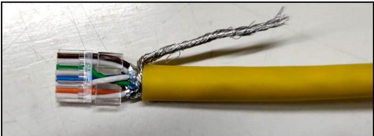
6. Push the cable in guide B to the end, cut off the protruding wire (here the assignment is according to T568B).
