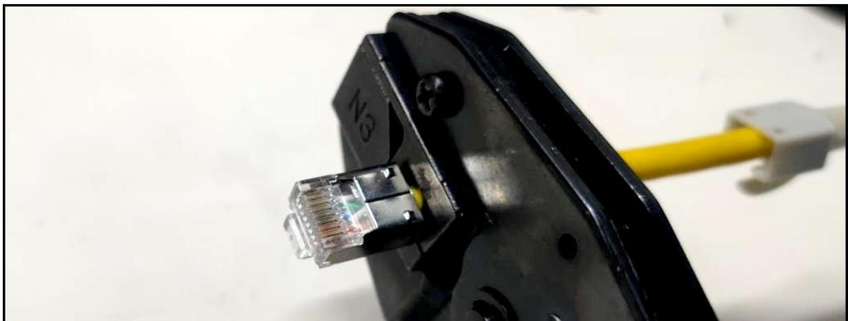
9. Crimp the dovetail clamp with the pliers tool.
