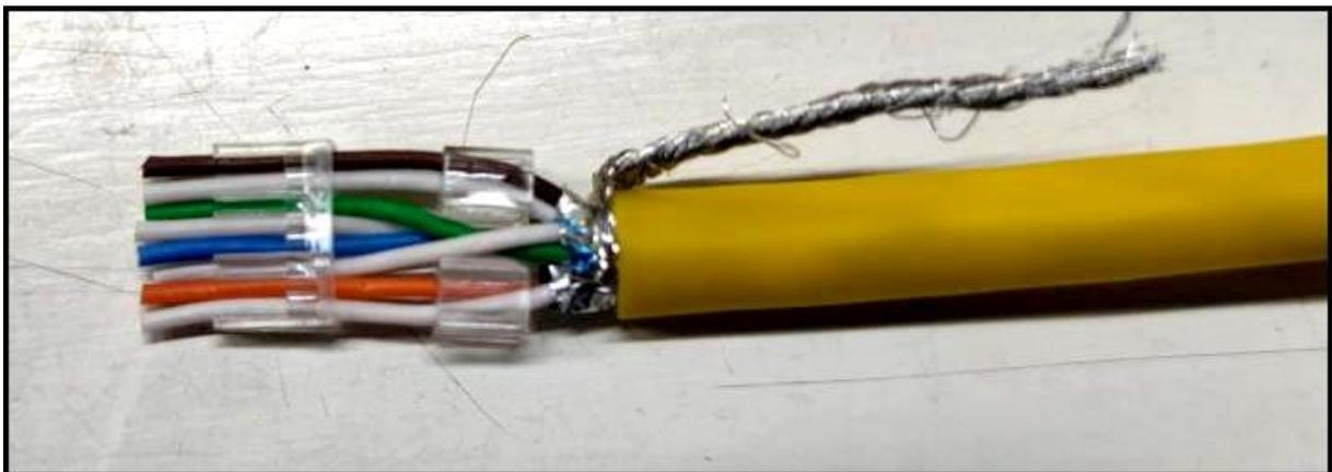
5. Insert the wires into cable guide B according to the T568B or T568A assignment.
