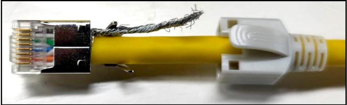
7. Insert the cable with both guides B and C into connector A.
