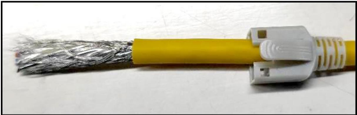
2. Feed the cable through sleeve D and strip approx. 30 mm of the outer sheath of the raw cable.
