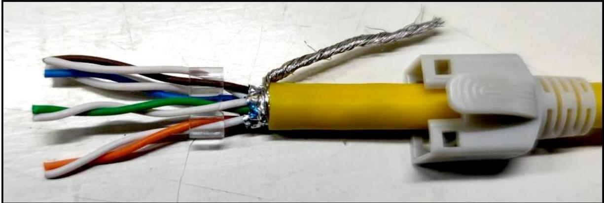
4. Insert each pair of cables into the 4 grooves of guide C (do not undo the twisting) (orange pairs and brown pairs in 2 of the grooves on the left and right) green pairs and blue pairs in the top and bottom 2 grooves)
