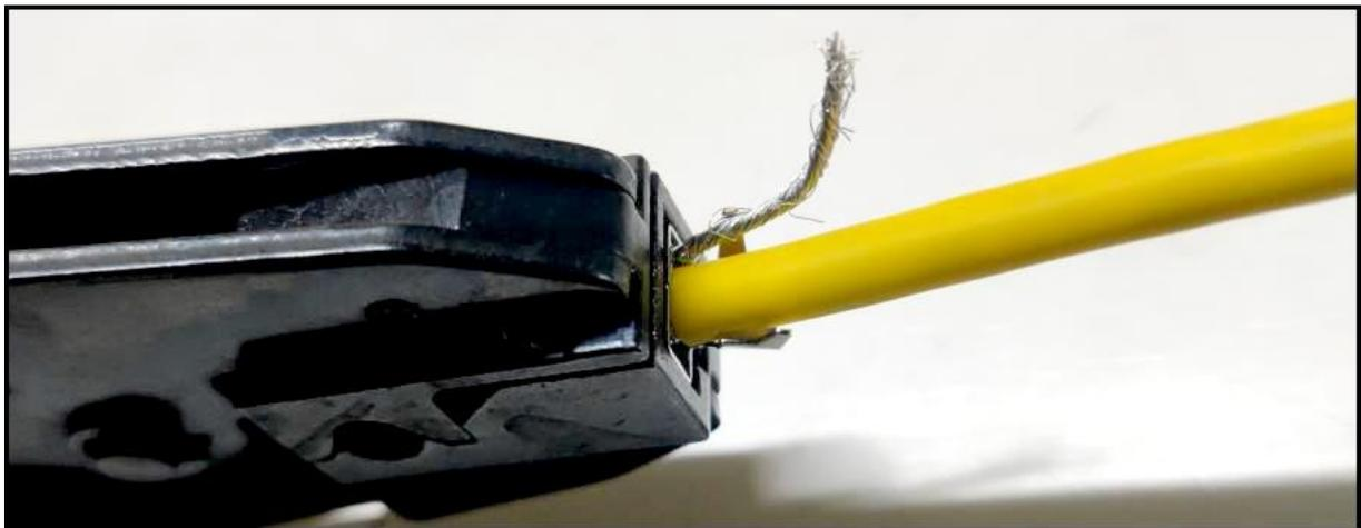
8. Crimp connector A with the crimping pliers.
