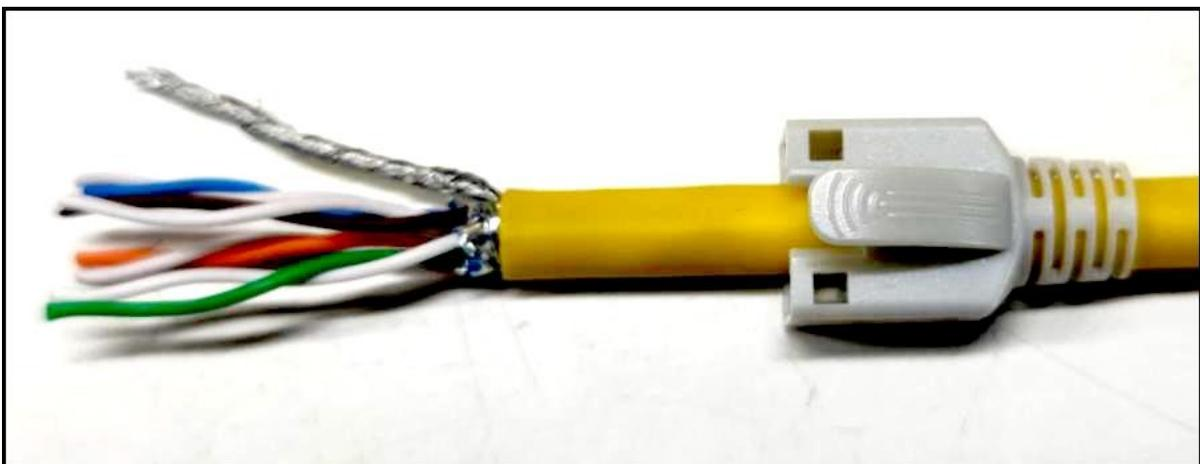
3. Twist the braid into a single wire and strip the insulation from the aluminium foil.
