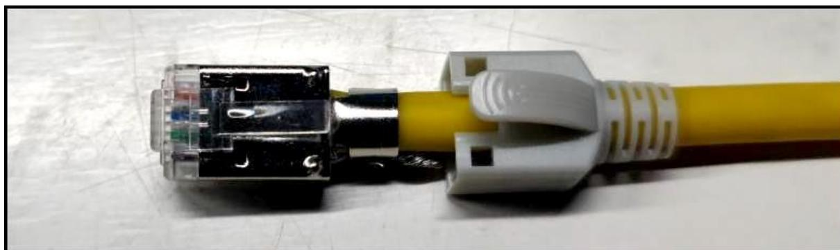
11. Push the sleeve D onto the plug A.
