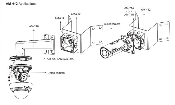
4. Secure the AM-714 conduit box to bracket using the M5 screws, washers, and hex heads. A hex crescent wrench is required.
