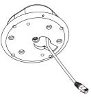
4. Pass cables through the waterproof rubber seal and complete all cabling requirements as documented in the camera QIG.
