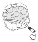
2. Install the bracket to the junction box using either the A or B holes.
