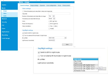
In the night mode, check if the input signals are correctly detected. You may simulate the night mode by blocking the IR unit's light sensor. Change the triggering parameters when necessary.
