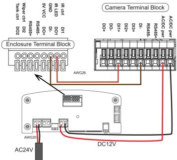
2. IR control by RS485 command Allow user to configure the RS485 command via camera web UI to cotrol IR on/of  $_{\rm f}$
