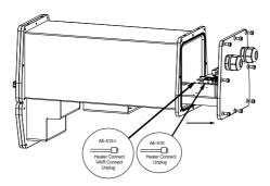
2. Prepare power wires, a ground wire, and a CAT5e Ethernet cable. Pass them through the PG16 waterproof connectors and its waterproof components.
