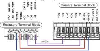
Below is a diagram for water tank and wiper control. The wiper can be started by manually triggering the Digital Output from the camera user interface.
