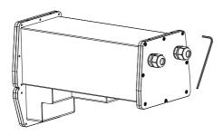
Slide out the rear cover plate of the housing, taking care to leave the sealing washer in its seating. Heater or wiper or VAIR connect need unplug.
