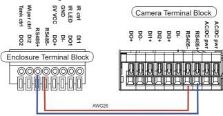
Note the wire gauge requirements for making the power connections. (24VAC 24W load)
