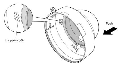
②Remove 1 stopper at a time while pushing down on the inner dome cover.
