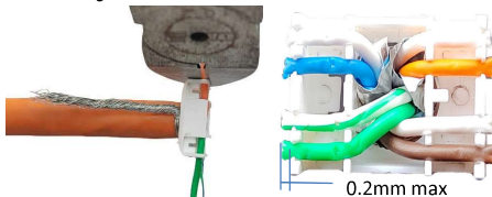
⑥. Allocate each conductor into proper slots on wiring cap by following color coding, then trim the the ends of conductors.
