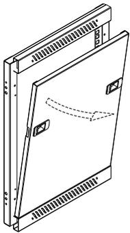
【1】 Remove ⑦ from ②, put them separate for the preparation of the frame assembly.
