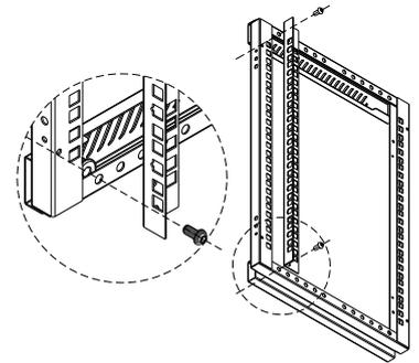
【3】 Fix 19" mounting rails to the first holes of top & bottom of side frames by 4sets of M5 screws.
