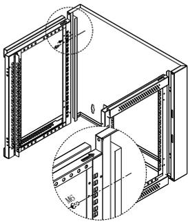
【4】 Install side frames to the grooves of back frame by 4pcs of M6\*12 screws (6pcs if more than 18U) as shown by the arrow in the picture, note 19" mounting rails are in the front side.
