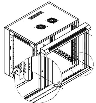
【6】 Install front frame by 4pcs of M6\*12 screws (6pcs of M6\*12 screws if more than 18U), refer to the picture.
