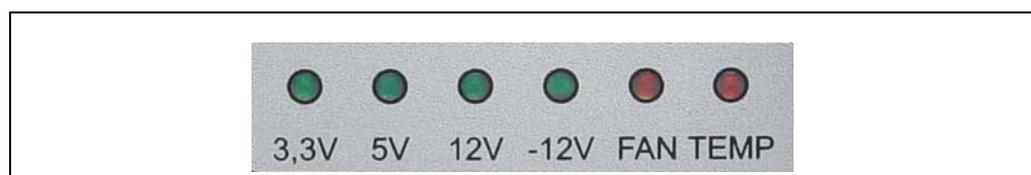
The Display Module is located at the upper front side of the subrack. 4 green LEDs signal the 4 VME64x voltages, two red LEDs signal over-temperature and fan fail events.
