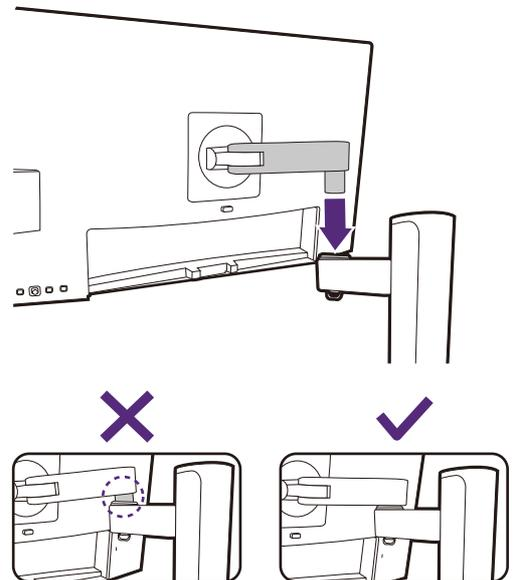
Raise the thumbscrew lid and tighten the thumbscrew as illustrated. Then push the lid back. If the upper arm is attached properly in the previous step, you will be able to tighten the thumbscrew.
