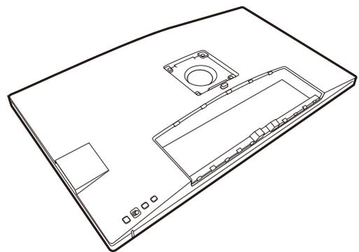
Use a cross-pointed screwdriver to release the screws that fixing the back cover to the monitor. The use of a magnetic-head screwdriver is recommended to avoid of losing the screws.
