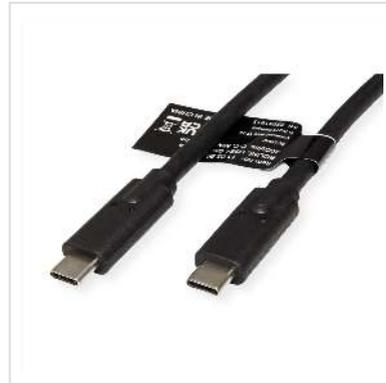
**High quality USB 4 Gen 2x2 cable with the reversible USB-C connector on both ends for data transfer rates of up to 20 Gbit/s and USB Power Delivery up to 20V / 5A.**
