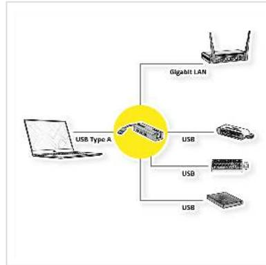
**With this converter you can connect your PC or notebook with USB 3.0 / USB 3.2 Gen 1 interface to a Gigabit Ethernet network.**
