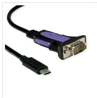
**A practical solution for using peripheral devices such as modems, digital cameras and printers equipped with serial interfaces together with notebooks or computers equipped with USB Type-C interfaces.**
