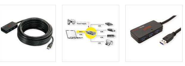
The handy hub with 10m long USB connection cable allows the connection of up to four USB peripherals at a greater distance from the PC. This makes the user almost independent of the location of the devices to be connected (e.g. printer). Power is supplied from the PC via the USB interface, but a power supply unit (5VDC, 3.5A) can also be connected as an option.
