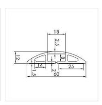
The cable bridge not only covers the cables lying on the floor, it also prevents tripping. The cable bridge has three cable passages that separate data and power supply cables - to prevent signal interference.
