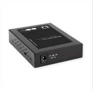
Fiber optic converters can be used to adapt different cabling within a LAN to create a functional network. Whether for converting fiber optics to a classic twisted pair network with a Mini-GBIC or for converting fiber optics to another fiber optic network with two Mini-GBICs. The ROLINE GigaBit converter offers both options.
