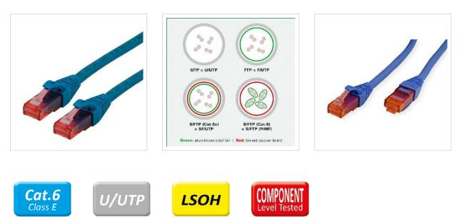
Patch cable for networking connections between devices. Prepared unshielded Twisted Pair cable with RJ-45 connectors on both ends. Durable due to moulded kink protection. Flexible cable, suitable for narrow bending. High quality plugs with gold plated contacts. Contact settings 1:1, in accordance with the EIA/TIA 568 standard. Construction: 4-pair stranded copper wire. Halogen-free, flame retardant, low smoke.
