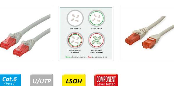
Patch cable for networking connections between devices. Prepared unshielded Twisted Pair cable with RJ-45 connectors on both ends. Durable due to moulded kink protection. Flexible cable, suitable for narrow bending. High quality plugs with gold plated contacts. Contact settings 1:1, in accordance with the EIA/TIA 568 standard. Construction: 4-pair stranded copper wire. Halogen-free, flame retardant, low smoke.
