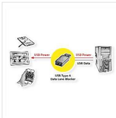
**The USB Type A Port Blocker blocks the data lanes of the used USB port and thus protects your end device from unwanted access or malware - nothing but power is transmitted. The solution is especially useful in foreign environments where USB sockets can be manipulated or hijacked comparatively easily, such as in hotels, or anchorage points like airports or train stations.**
