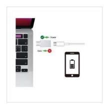
This USB Type A Male to USB Type C Femal port blocker blocks the data lines of the USB port and therefore protects your end device from unwanted access or malware - only power is transmitted. This solution is particularly useful in environments where USB ports are easy to manipulate or hijack, such as hotels, airports, train stations, fairs or other public premises.
