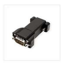
To connect serial devices to a RS232 port on your PC with electrical isolation
