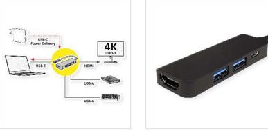
Connect your Macbook, Ultrabook, Notebook/Laptop or PC with USB Type C interface to an HDMI display or projector (with a maximum resolution of up to 3840x2160 @30Hz) and another device, e.g. an external harddisk, to the additional USB Type A Port, while charging your device simultaneously over the Type C PD port!
