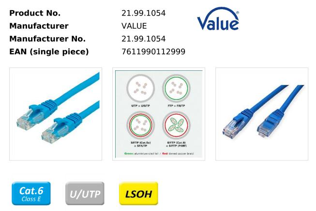
Patch cable for networking connections between devices. Prepared unshielded Twisted Pair cable with RJ-45 connectors on both ends. Durable due to moulded kink protection. Flexible cable, suitable for narrow bending. High quality plugs with gold plated contacts. Contact settings 1:1, in accordance with the EIA/TIA 568 standard. Construction: 4-pair stranded wire. Halogen-free, flame retardant, low smoke.
