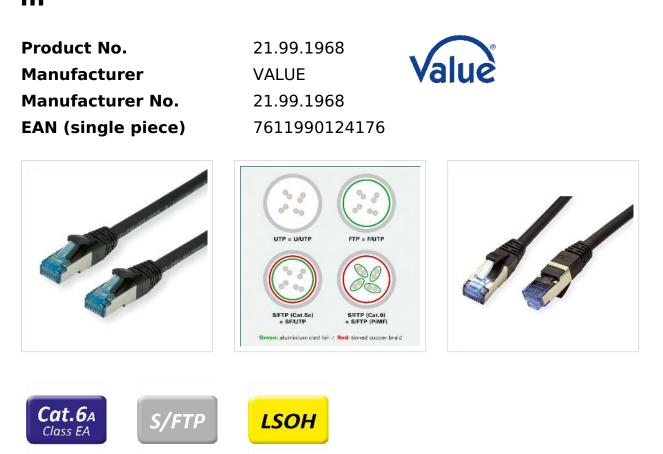
The cheap solution for data transfer rates of up to 10 Gbit/s and a bandwidth of 500 MHz. Patch cable for networking connections between devices. Prepared shielded Twisted Pair cable (PiMF) with RJ-45 connectors on both ends. Durable due to moulded kink protection. Flexible cable, suitable for narrow bending. Impedance: 100 Ohm. Contact settings 1:1, in accordance with the EIA/TIA 568 standard. Construction: 8 lines, pairs shielded with aluminium foil, complete braided shielding.
