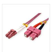
OM4 fiber for existing 1 and 10 Gbit/s applications as well as future 40 and 100 Gbit/s systems. Allows extended reach upwards of 550 meters at 10 Gbit/s for ultra long building backbones and medium length campus backbones. With an laser bandwidth of 4700 MHz-km (more than double the IEEE requirement for 10 Gbit/s 300 meter support), the OM4 fiber is also especially well suited for shorter reach in data centers and high performance computing applications.
